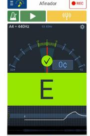
The needle is centered, a check sign is displayed and the screen turns green – it means you're good to go!
