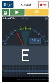
If the needle is situated on the left side it means the E string is too low. In this case we need to tighten the string.
